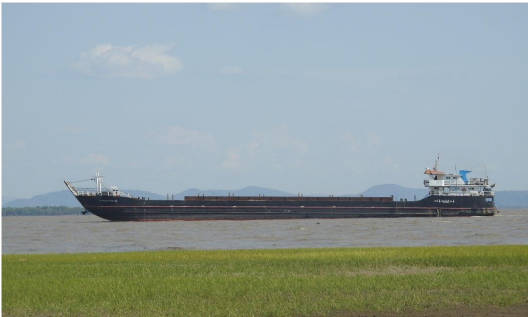
Fig: 7 Sand mining vessel at Thanlwin river mouth
